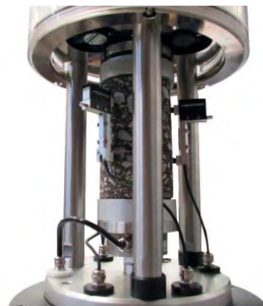
Asphalt specimen with on-specimen LVDTs and load cell
